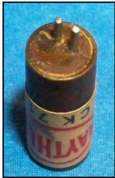
Transistor Size (1/4"OD X 5/8"H) No Date Code Stamp
