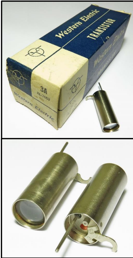
Size: Approx 1 3/16" L X 7/16" OD Date Code: 7603 on box Date Code: 369 stamped on device
