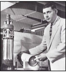
Shown at top is a 1958 photo of George Ludwig in Pasadena with the Explorer I backup satellite. (Photo courtesy of George Ludwig). The second photo is also from 1958 and shows Ludwig holding his newly designed data recorder which performed flawlessly in Explorer III and which contributed to the discovery of the Van Allen radiation belts. The Explorer III instrumentation package is at left in the photo. (AP Wire Photo).
