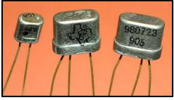
George Ludwig selected early silicon transistor types for use in the Explorer satellite cosmic ray package. The Texas Instruments 2N33X series, shown above at top, was used in the GM scalar circuits for Explorer I and IV. The TI 900 series transistors shown above was used for the scalar circuits in Explorer III. Shown at right is an ad from the Feb 13, 1959 issue of Electronics magazine showing the 2N33X transistors mounted on the GM scalar circuit board designed and built by Ludwig.
