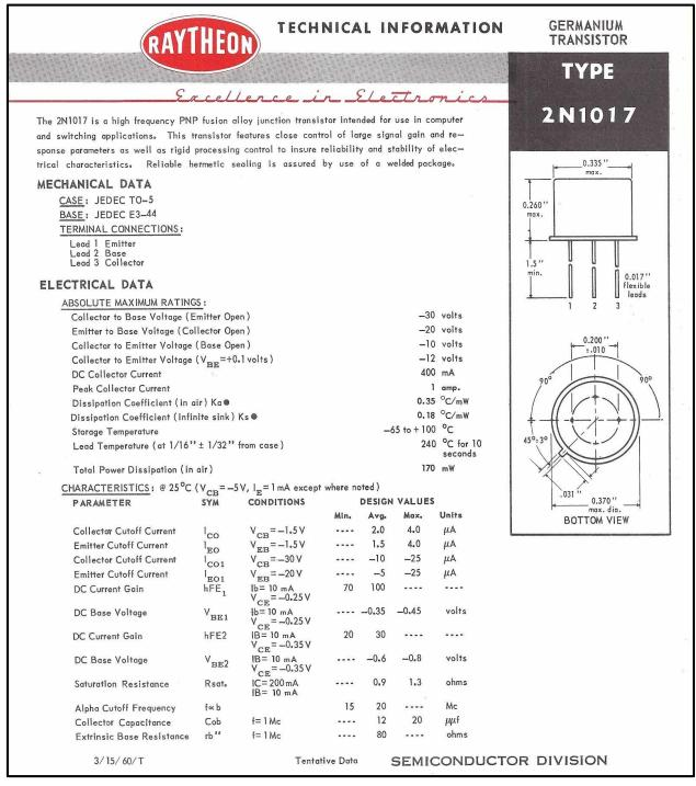
Raytheon Computer Transistor Data Sheet: Above is an example of a typical Raytheon transistor "spec sheet" from the 1950s/1960s - this "spec sheet" documents the Tentative performance parameters of the 2N1017 germanium computer transistor. By this time, the standard TO-5 case style was used for the 2N1017, although an earlier 1958 Raytheon "spec sheet" lists the less common TO-9 case.
