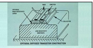
The Sylvania epitaxial structure uses a main collector body region of very low resistivity material with a thin epitaxially grown high resistivity region. This permits a significant reduction of collector series resistance (saturation voltage) and an increase in switching speed (less excess stored charge). Also collector capacitance is reduced through the use of the epitaxially grown high resistivity region.
