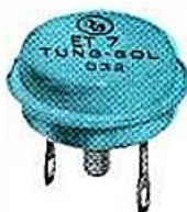
ET-7 AF High Power Amplifier PNP
