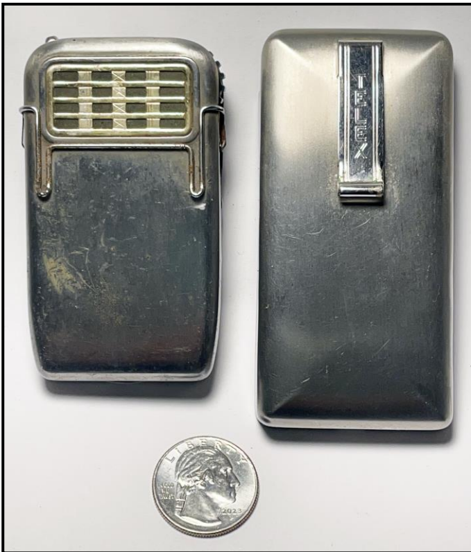
Historical Examples of the First Use of Transistors in Hearing Aids in the Current Transistor Museum Collection
